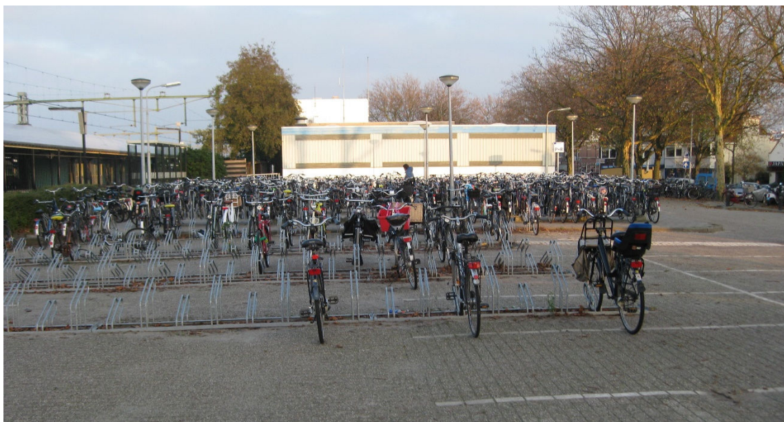
2.7 Bad example of bike racks: no possibility to secure the bike properly
