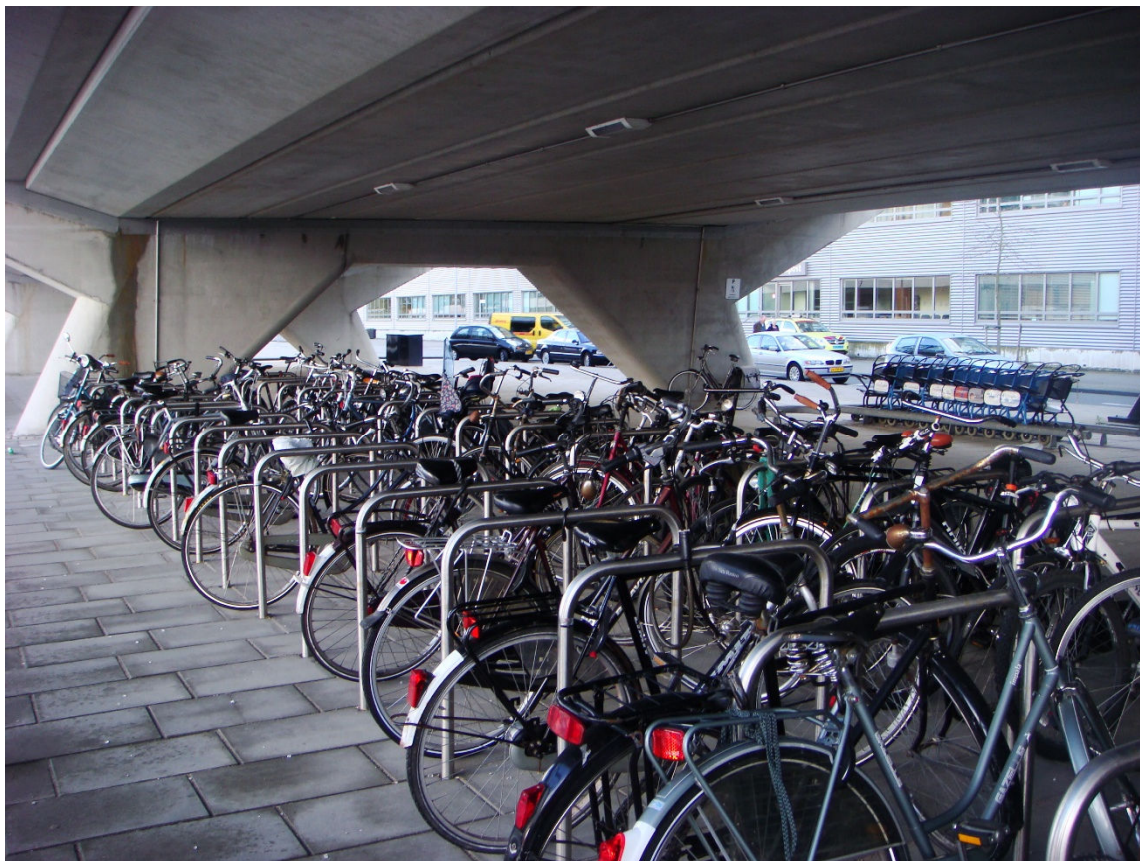
2.8 Good cycling racks provide an extra 'fastening feature' to lock both the wheels and the frame to an object
