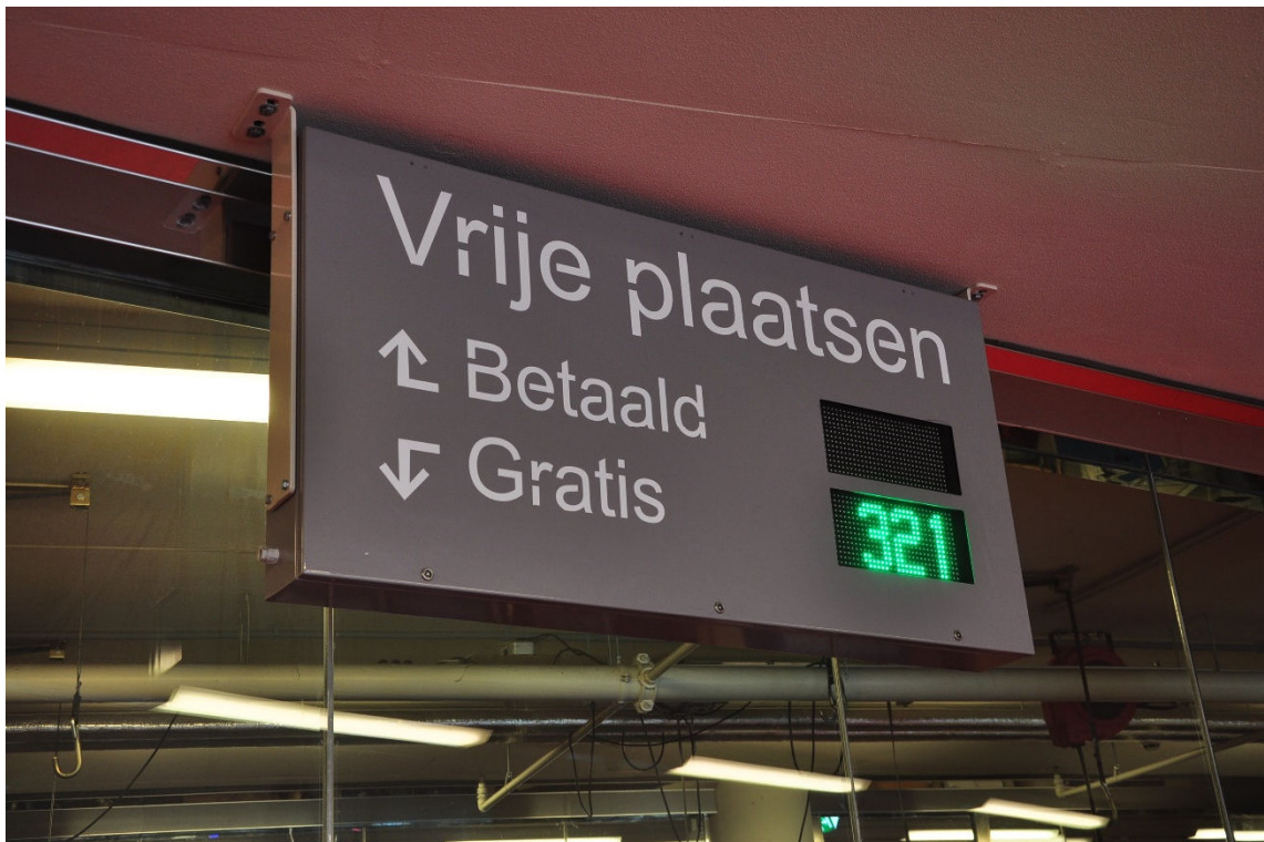
2.13 Wayfinding system indicating available places in bike racks at a bike parking in the Netherlands. This system is now used more and more within big bike parkings and offer users the possibility to find free parking places quicker.
